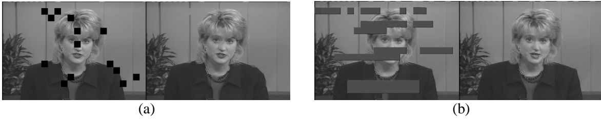
Figure 1. (a) Spatial error concealment. Left: Missing macroblocks. Right: Recovered errors. (b) Temporal error concealment. Left: Missing macroblocks. Right: Recovered errors.
