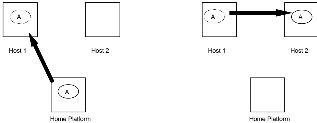
Figure 3: Movement of agent from home platform to host 1 and 2 for data collection and information assurance
