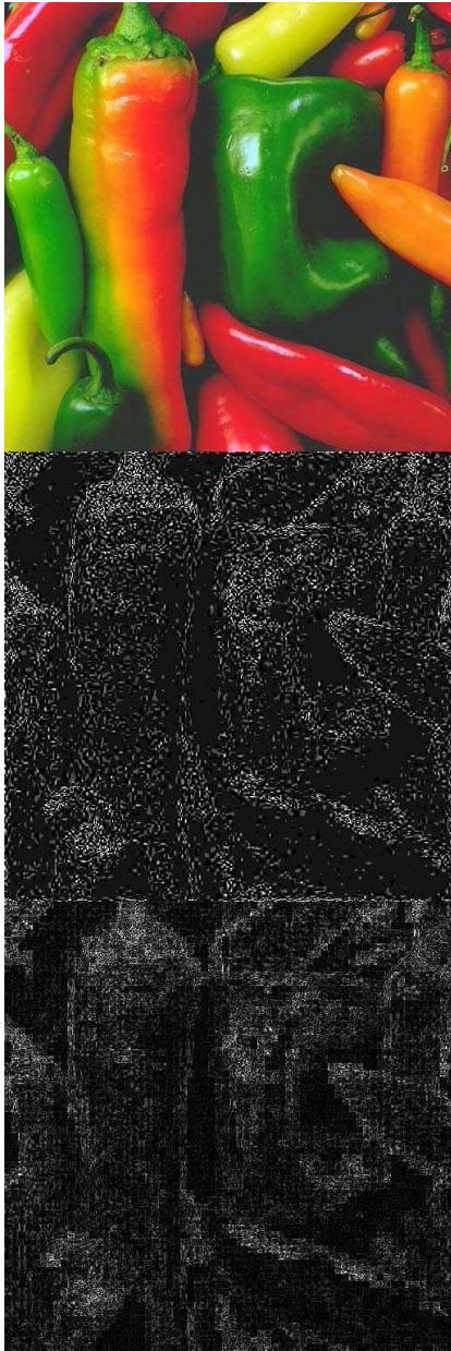
Figure 5. Top: image marked with IA-W; center: the IA-W watermark; bottom: the IA-DCT watermark.
