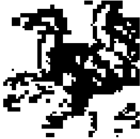
Figure 8: Final suitability map for sample image. The regions shown in white are the ones that are labeled as unsuitable for embedding.
