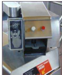
Fig. 6. Two-finger Geometry System Implemented by Disney Inc. (Levin, 2001).
