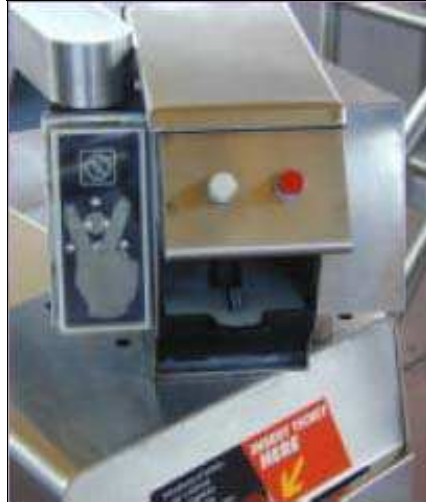
Fig. 9. Two-finger Geometry System Implemented by Disney Inc. (Levin, 2001).
