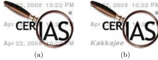
Fig. 2. Logo images watermarked with ImageMagick TM : (a) time only watermark (b) watermark with both time and mnemonic, in this image the mnemonic is Kakkajee .
