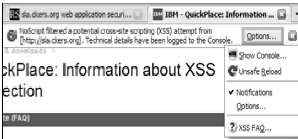
Figure 3.2 XSS filtering in NoScript. Adapted from “NoScript - JavaScript/Java/Flash blocker for a safer Firefox experience! - features – InformAction” by G. Maone, n.d. b, retrieved from http://noscript.net/features
