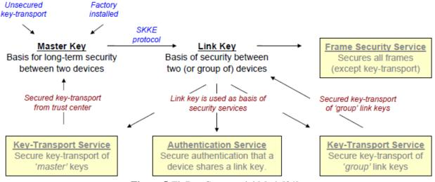
Figure 5:ZigBee Commercial Mode[34]
