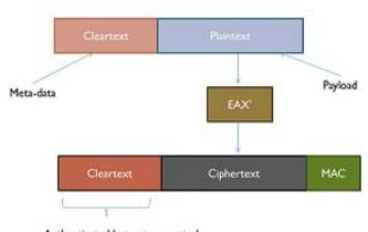
Authenticated but not encrypted Figure 6: EAX' Encryption
