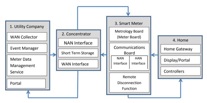
**Figure 1:**The Advanced Metering Infrastructure (AMI) consisting of four main logical components:1.the Utility Company, 2. the Concentrator, 3. he Smart Meter, and 4. the Home
