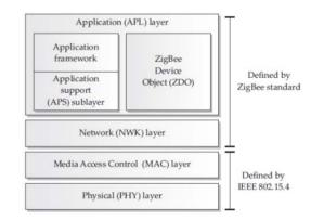
Figure 3: ZigBee Protocol Stack [34]
