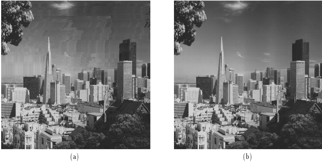
Figure 3: Comparison of the “San Francisco” image compressed by PMIC: (a) with constant D and compression ratio 7.5; (b) variable D and compression ratio 8.3.
