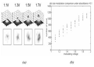
Figure 4 Dot size and laser intensity modulation
