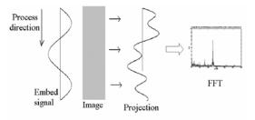
Figure 2 Embedding and detecting extrinsic banding signal
