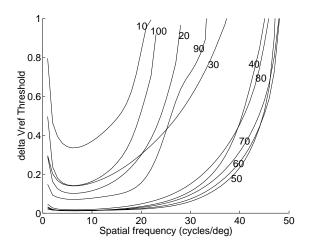
Figure 8 Mapping between the  $\Delta V$  threshold and the spatial frequency for difference desired gray levels
